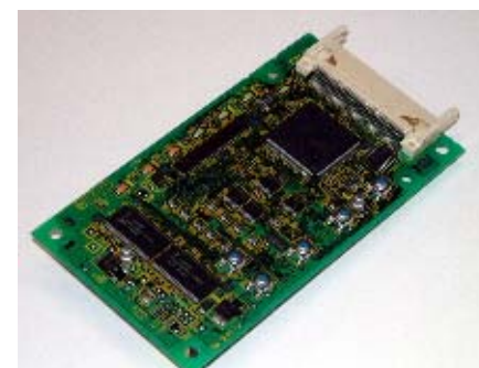
Prototype board for vending machines, based on picoJava™-II LSI (Fuji Electric Co., Ltd.)
