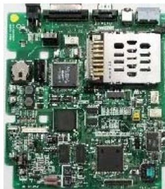
Trial production board for net appliance based on the PersonalJava™/picoJava™-II (Fujitsu Ltd.)
