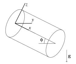
Using orthogonal coordinates with the x-axis aligned with the axis of the tube and the y-axis horizontal as indicated, find a solution for the flow along the tube under the assumptions that the flow is steady and uniform along the tube and the fluid fills the tube. Find the total flow rate of fluid out of the pipe.
